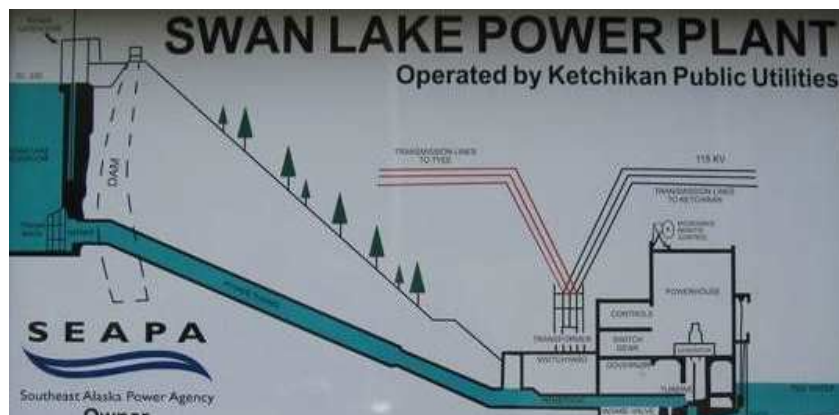
Dam 174' high x 430' wide Spillway 15' high x 100' wide
